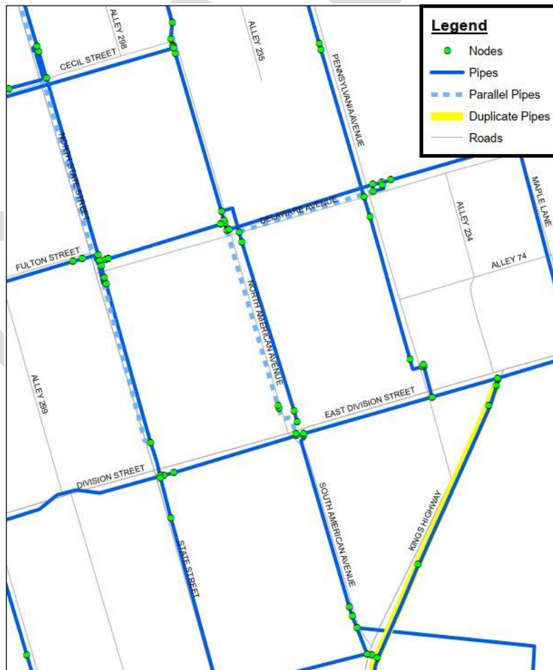
Figure 6.1 – In Service Parallel Pipes
